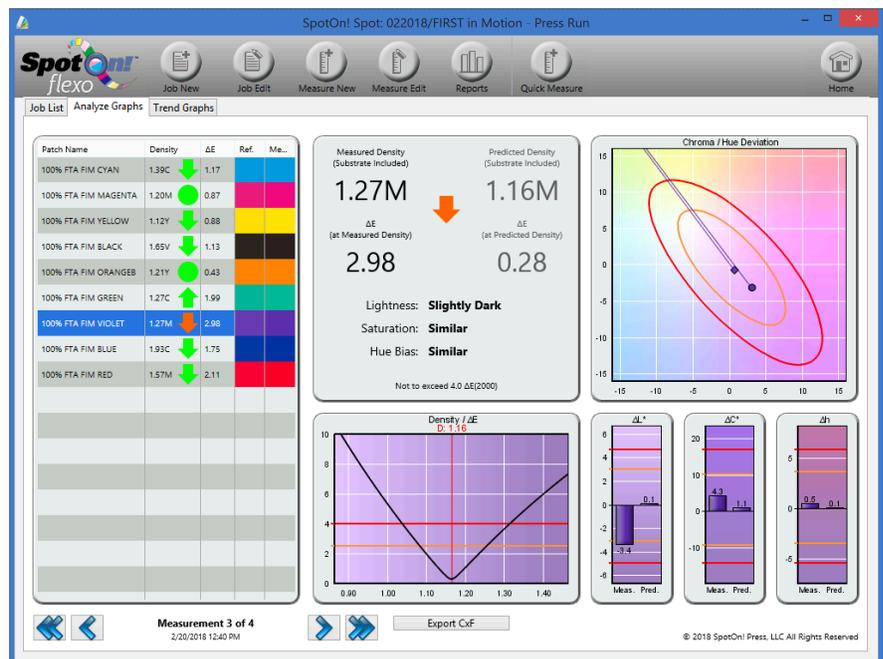
This chart provides the press operator the range of ink density that can be run (1.08 – 1.26) and still maintain an acceptable color match of under 2.5 dE00. This is new information for the press operator and changes the way we look at the color approval process. With this data, the press operator or quality control manager can objectively approve color on press based on colorimetric data.
