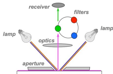
In the press room, a densitometer can monitor the ink film thickness being applied to the substrate or media. An increase in density results in a darker color and decrease in density results in a lighter color.
