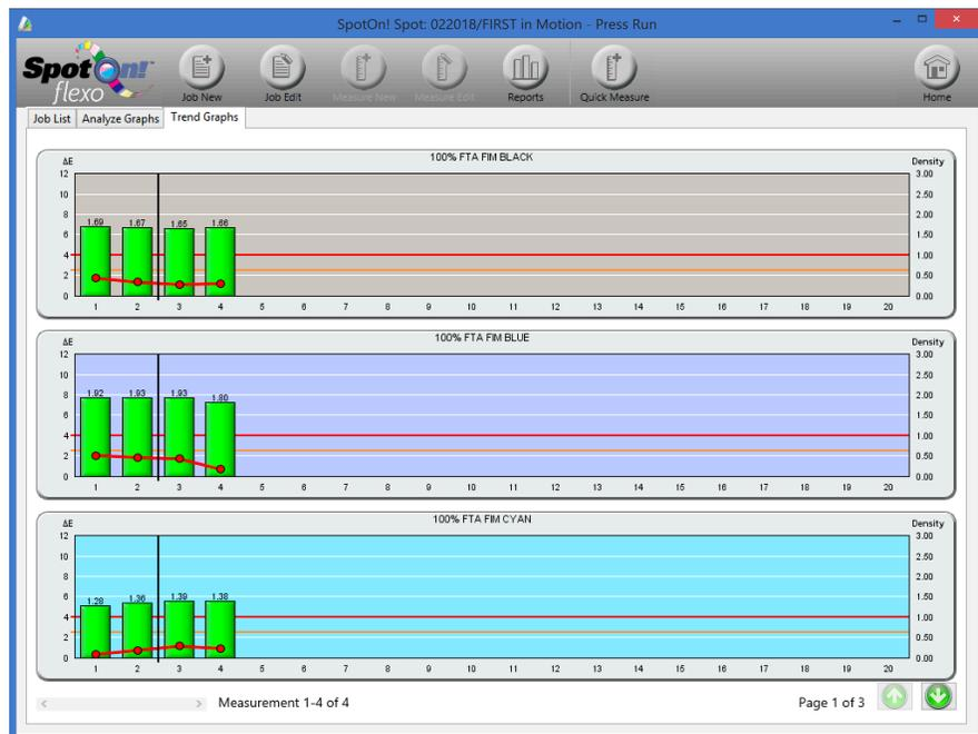
This job-related metadata can contain items such as the type of ink, plates, mounting tape, substrate, and anilox rolls being used. This data can then be used to create Reports of the press runs.
